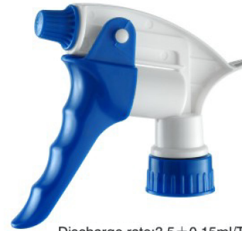
Discharge rate:3.5±0.15ml/T Closure:28/400,28/410,28/415 Function:SPRAY-STREAM-OFF QTY:300PCS/CTN Meas:45x39x57CM
